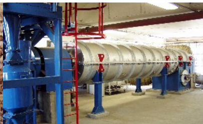
3R zero emission biochar production unit
